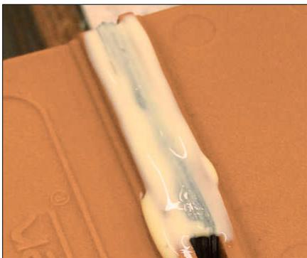
When the glue has dried, remove the “notepad” from the clamp and trim off any excess glue. Wood glue has enough “give” that it will allow the “notepad” to be flexible and individual pieces can easily be removed as you need them.
